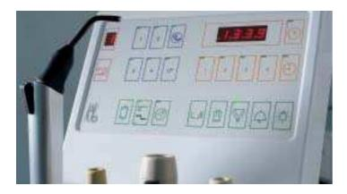
Membrane switches excel due to their space-saving and compact construction, safe function, and last but not least by insensitivity to humidity and soiling. The boundless design possibilities are a further consideration.
